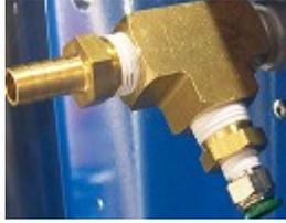
Attach other end of hose to inlet on the storage tank. **Do not tee this hose with the outlet of the regulator from a delivery stand. Causing back pressure in this manner will destroy the membranes.**
